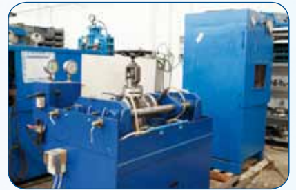
HYDRO - PNEUMATIC TEST UP TO 1000 bar
