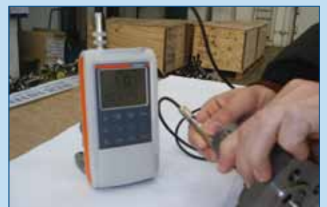
FERRITESCOPE FISHER FOR FERRITE DETERMINATION
