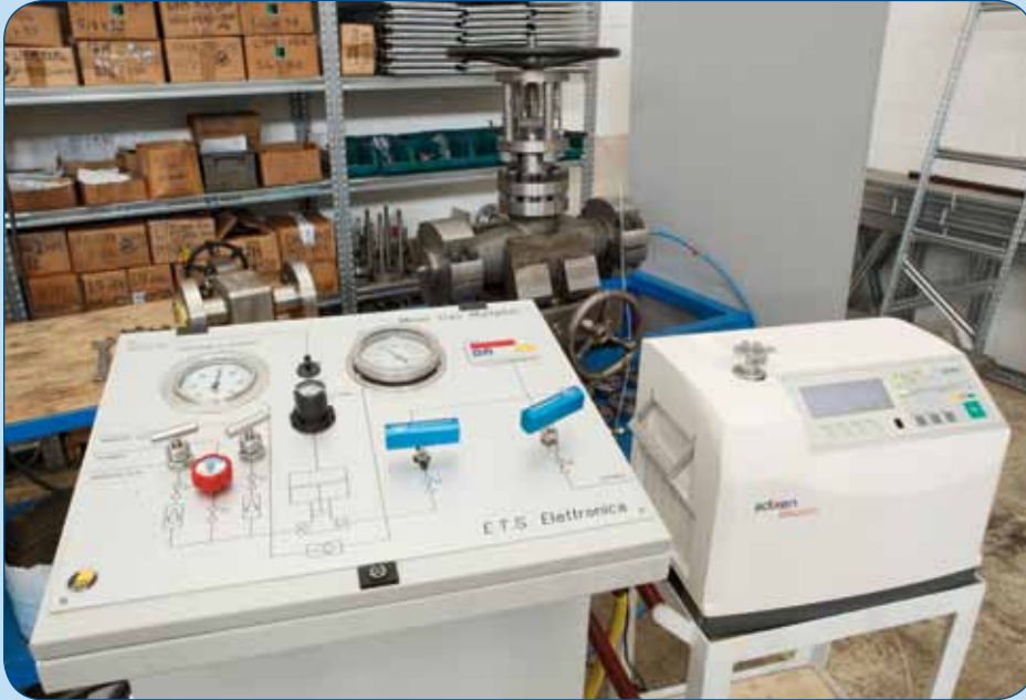
HP GAS TEST FACILITY AND FUGITIVE EMISSION HELIUM LEAK DETECTOR TEST
