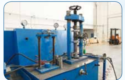
HYDRO - PNEUMATIC TEST UP TO 600 bar
