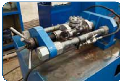
HYDRO - PNEUMATIC TEST UP TO 600 bar FOR CHECK VALVES
